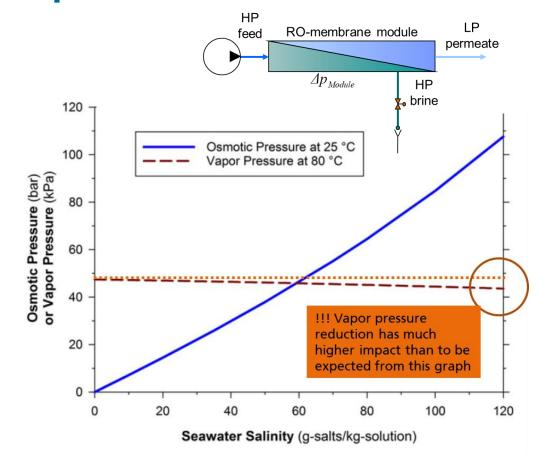
Brine treatment needs extremely high pressure! Therefore usually thermal distillation is applied
