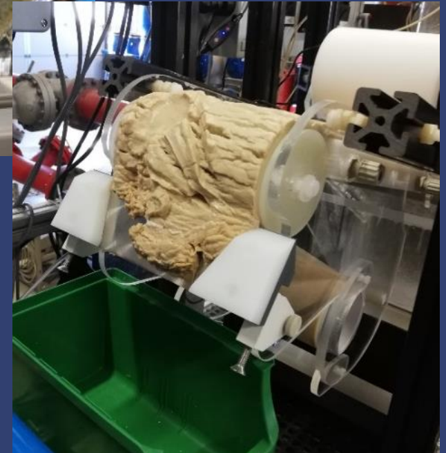
Band filter for continuous precipitate extraction
