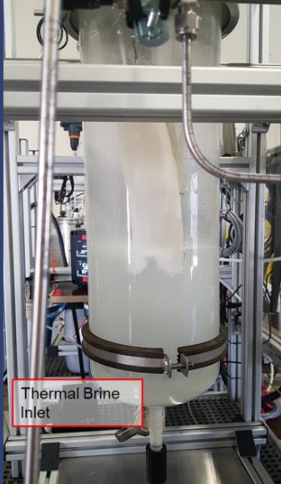
Thermal brine inlet reactor
