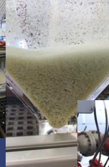
Settling of Ca-Si precipitates
