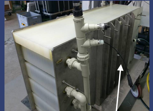
MD-membrane stack for post concentration
